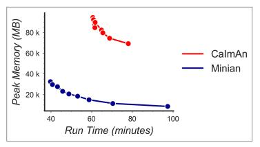
**Figure 19.** Tradeoff between run time and memory usage. Simulated data with 500 cells and 28,000 frames were processed through Minian and CalmAn with different numbers of parallel processes. We varied the number of parallel processes from 2 to 10, and the resulting memory usage is plotted as a function of run time. For both pipelines, the curve takes a hyperbola shape, showing the tradeoff between run time and memory usage.
