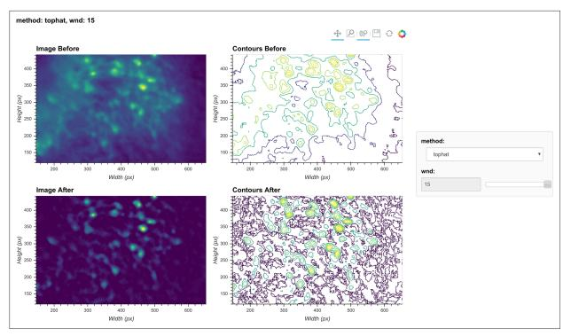
**Figure 6.** Visualization of background removal. Here, a single frame from the data is passed through background removal, and both the image and a contour plot are shown for the frame before and after the process. The plots are interactive and responsive to the slider of the window size on the right, thus the effect of different window sizes for background removal can be visualized.
