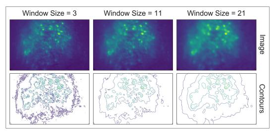
**Figure 5.** Effect of window size on denoising. One example frame is chosen from the data, and the resulting images (top row) and contour plots (bottom row) are shown to demonstrate the effect of window size on denoising. Here, a window size of 11 (middle column) is appropriate while both smaller and larger window sizes result in artifacts.
